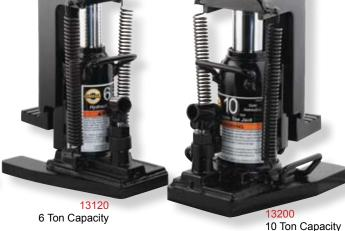
Minimum Maximum Minimum Maximum Base Base Hydraulic Model Capacity Toe Toe Head Head Size Size G.W. Lifting Height Height Height Width Height Length 13060 3 Ton 5/8" 5-3/4" 9" 14-1/8" 8-5/8" 7-1/2" 39 Lbs. 13120 6 Ton 7/8" 6" 10-1/2" 15-5/8" 5-1/8" 11" 7-1/2" 55 Lbs. 13200 10 Ton 1-1/8" 6-1/4" 11" 16-1/8" 11-5/8" 9-1/4" 86 Lbs.
